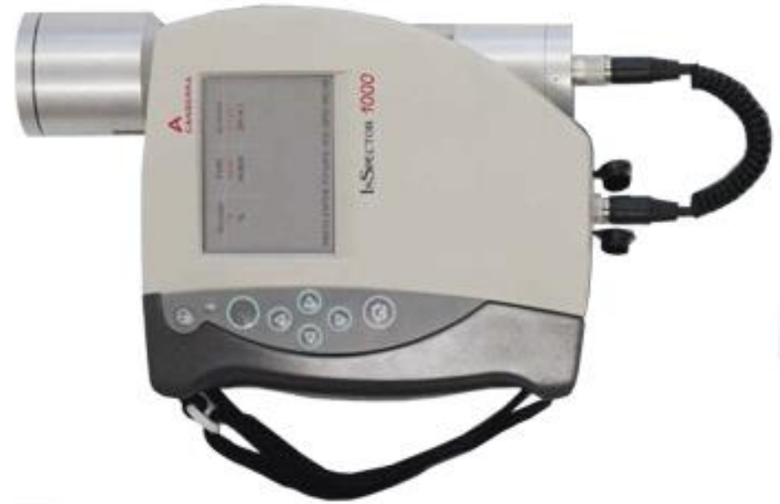
Radiometer-spectrometer (identifier) - Canberra InSpector 1000.
