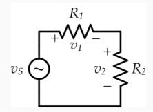
$$v_1 = v_s \frac{R_1}{R_1 + R_2}$$
