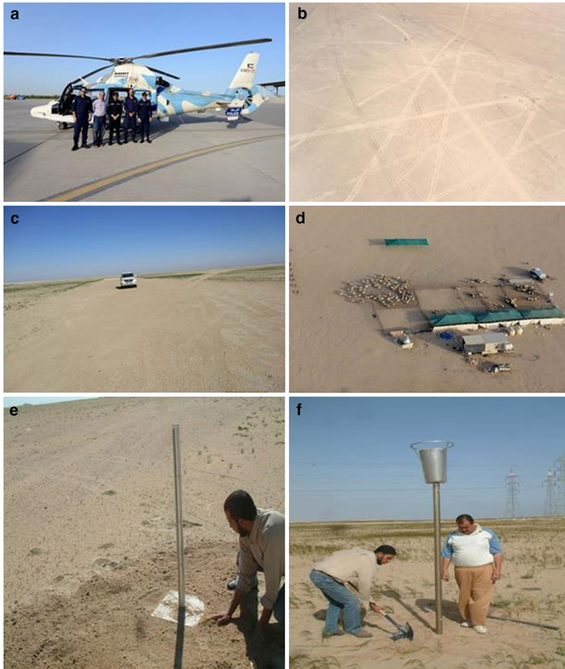
Fig. 2 Aerial photos were captured using helicopter trips ( a ) for off-road vehicle tracks ( b , c ) and grazing point ( d ), traps for monitoring aeolian sand ( e ) and dust ( f )
