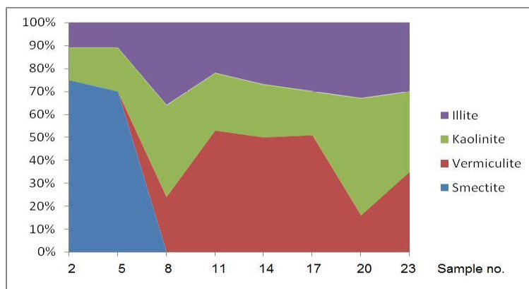
Fig. 6. Lateral distribution of clay minerals in sediments from Sharm Obhur.
