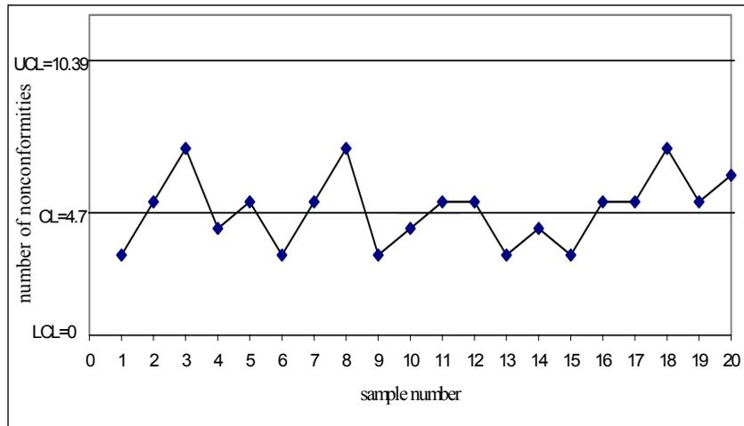
Figure 7: Control Chart for Plug-Assist process in normal operation conditions. CL =4.7, UCL =10.39, and LCL =0.
