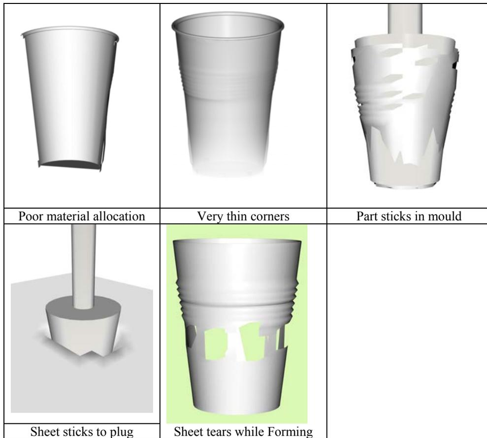
Figure 5: Illustrations of the detected defects in the factory.
