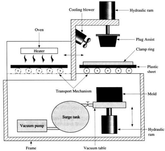
Figure 4: Illustrative drawing for Plug-Assist machine.
