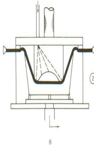
Figure 2: The forming and blowing phase.
