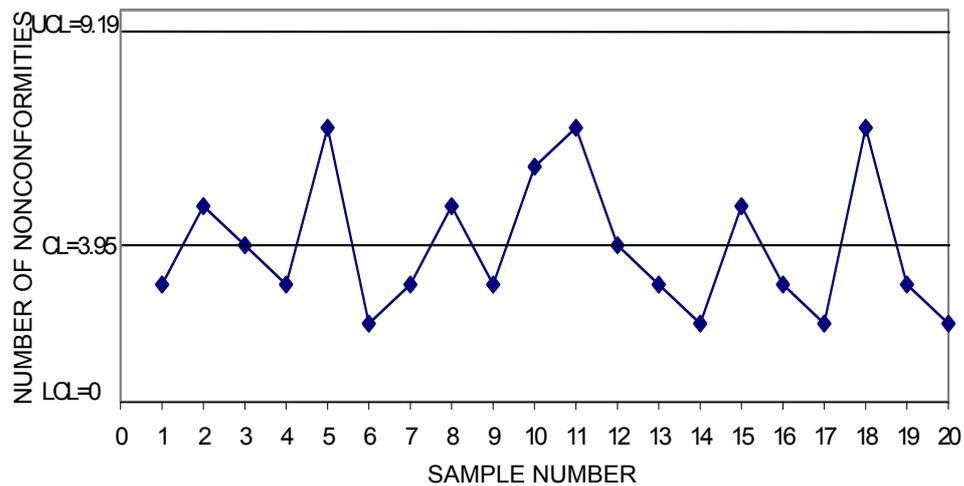
Figure 11: Control Chart for Plug-Assist process in normal operation conditions after modification. CL =3.95,UCL =9.19, and LCL=0
