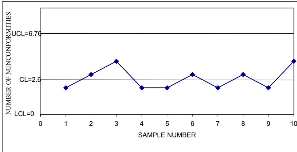
Figure 10: The control chart just at the beginning of the manufacturing process after modification. CL =2.6,UCL =6.76, and LCL =0.0
