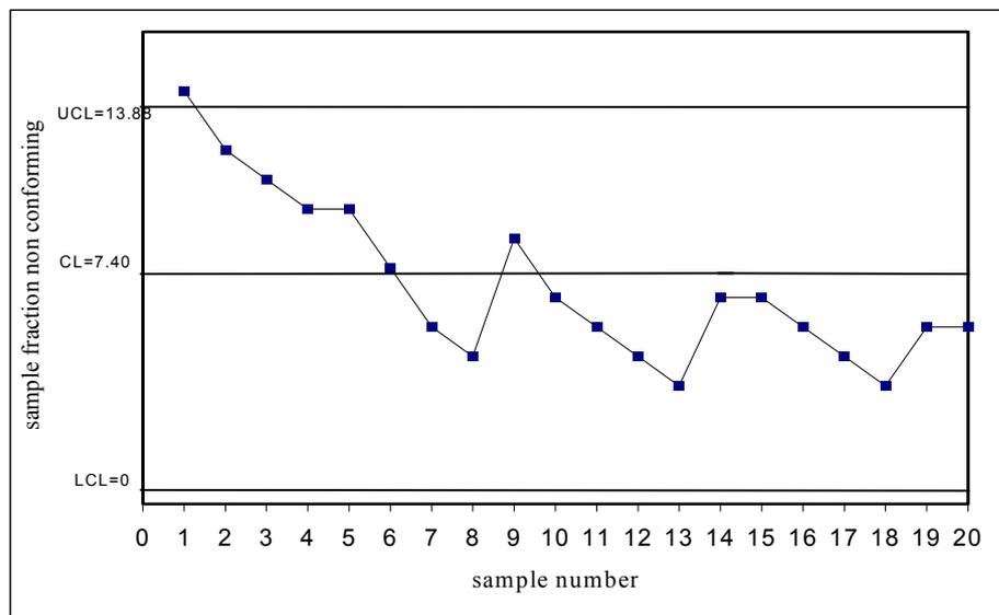
Figure 6: The np-control chart just at the beginning of the manufacturing process. CL (center line)=7.4, UCL (upper control limit)=13.88, and LCL (lower control limit)=0.92
