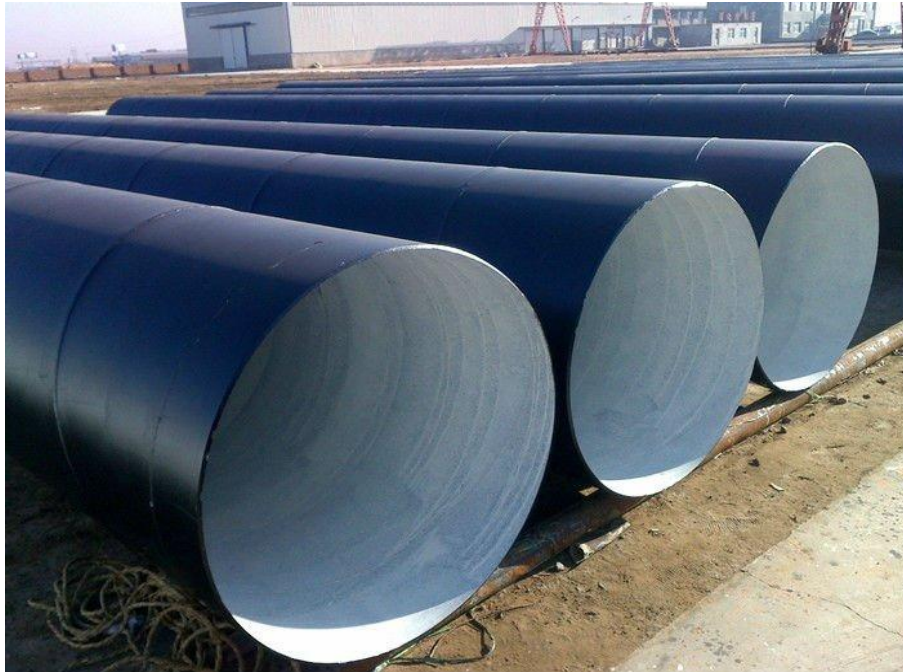
Fig. 6, Coating of outside surface of pipeline with coal tar + epoxy
