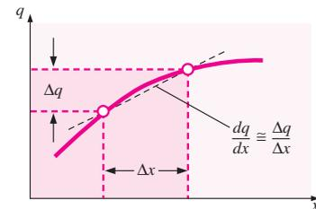
**FIGURE 4-11** A first-order finite difference approximation for derivative  $dq/dx$  is simply the change in dependent variable ( $q$ ) divided by the change in independent variable ( $x$ ).
