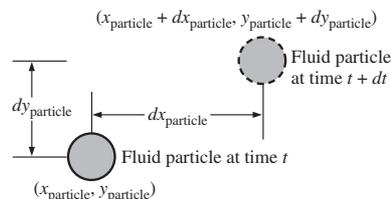
**FIGURE 4-7** When following a fluid particle, the  $x$ -component of velocity,  $u$ , is defined as  $dx_{\text{particle}}/dt$ . Similarly,  $v = dy_{\text{particle}}/dt$  and  $w = dz_{\text{particle}}/dt$ . Movement is shown here only in two dimensions for simplicity.
