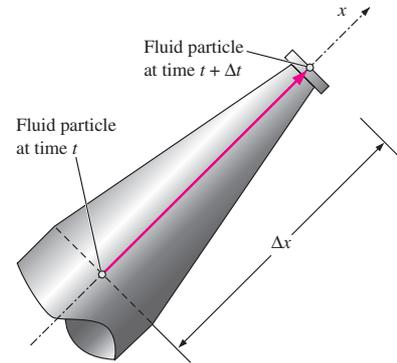
**FIGURE 4-10** Residence time  $\Delta t$  is defined as the time it takes for a fluid particle to travel through the nozzle from inlet to outlet (distance  $\Delta x$ ).
