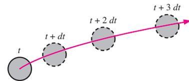
**FIGURE 4-12** The material derivative  $D/Dt$  is defined by following a fluid particle as it moves throughout the flow field. In this illustration, the fluid particle is accelerating to the right as it moves up and to the right.
