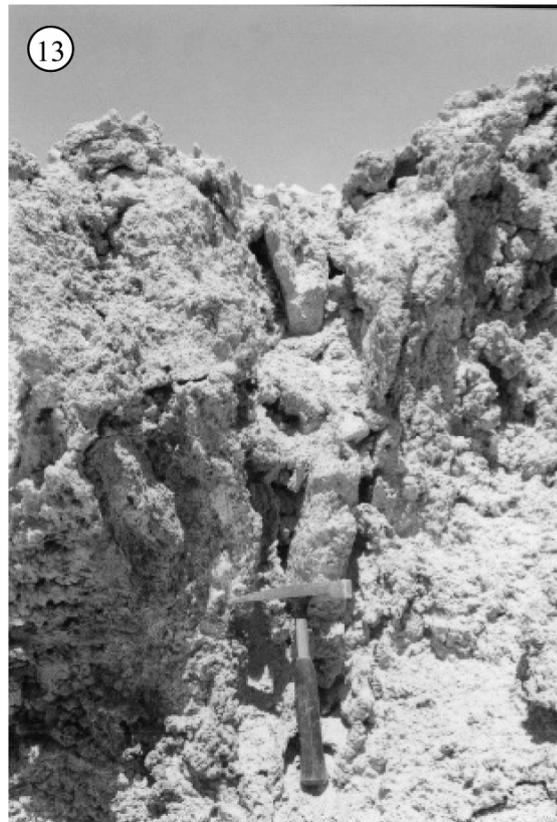
Fig. 10: Resistant gravel cemented with gypsum crust over the marl layer.
