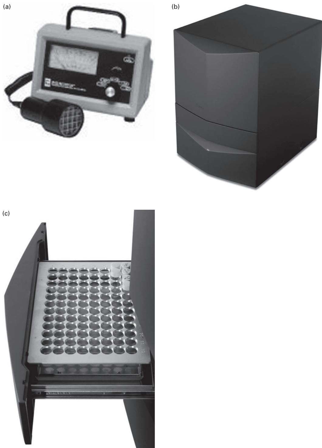
Fig. 14.4 (a) Geiger-Müller bench monitor; (b) liquid scintillation counter; (c) sample rack for liquid scintillation counter. (Reproduced with permission from LabLogic; instrument shown is the Hidex 300SI.)
