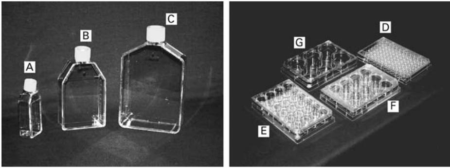
Fig. 2.2 Tissue culture plastics used generally for cell culture. (A–C) T-flasks; (D–G) representative of multi-well plates. (A) T-25 (25 cm<sup>2</sup>), (B) T-75 (75 cm<sup>2</sup>), (C) T-225 (225 cm<sup>2</sup>), (D) 96-well plate, (E) 24-well plate, (F) 12-well plate and (G) 6-well plate.
