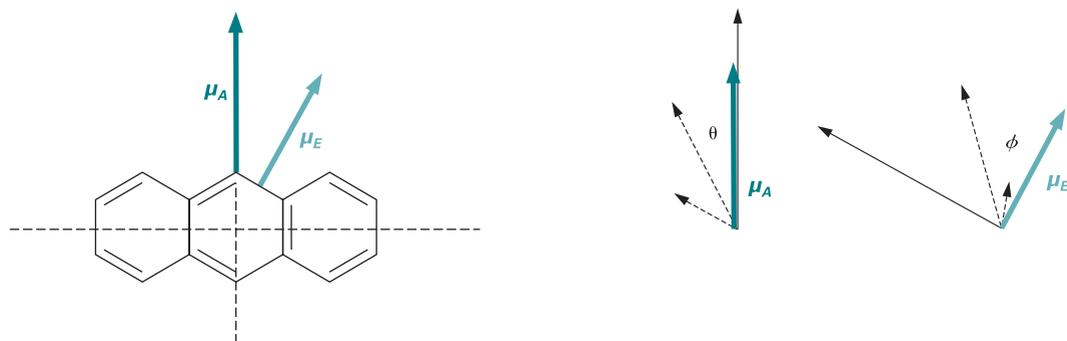
Fig. 12.15 Absorption dipole moment  $\mu_A$  (describing the probability of photon absorption) and transition dipole moment  $\mu_E$  (describing the probability for photon emission) for any chromophore are usually not parallel. Absorption of linearly polarised light varies with  $\cos^2\theta$  and is at its maximum parallel to  $\mu_A$ . Emission of linearly polarised light varies with  $\sin^2\phi$  and is highest at a perpendicular orientation to  $\mu_E$ .
