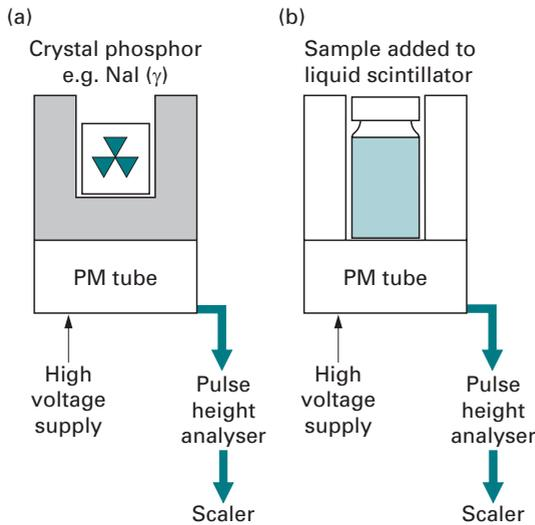
Fig. 14.6 Diagrammatic illustration of (a) solid and (b) liquid scintillation counting methods.
