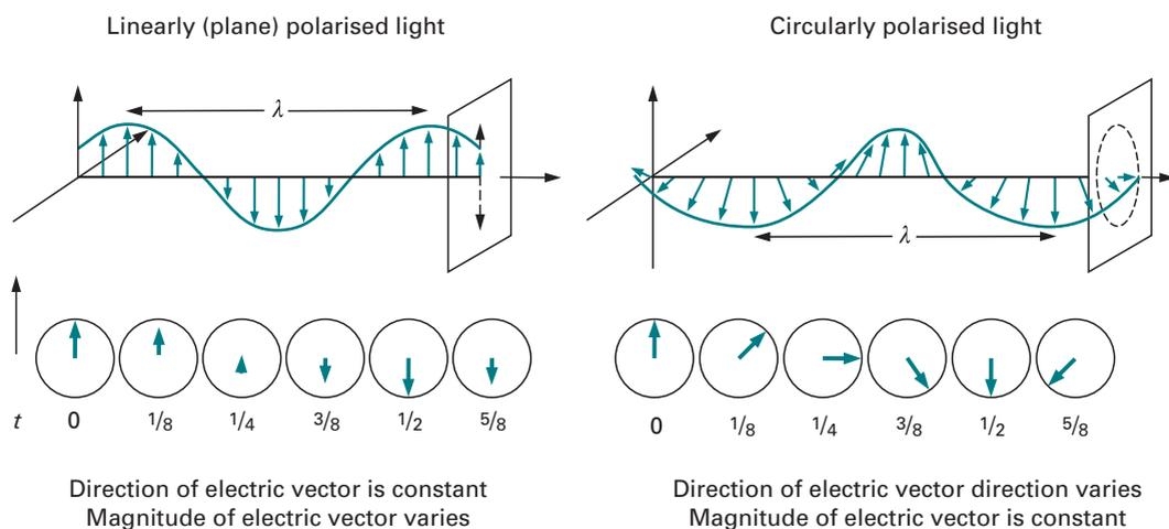
Fig. 12.16 Linearly (plane) and circularly polarised light.
