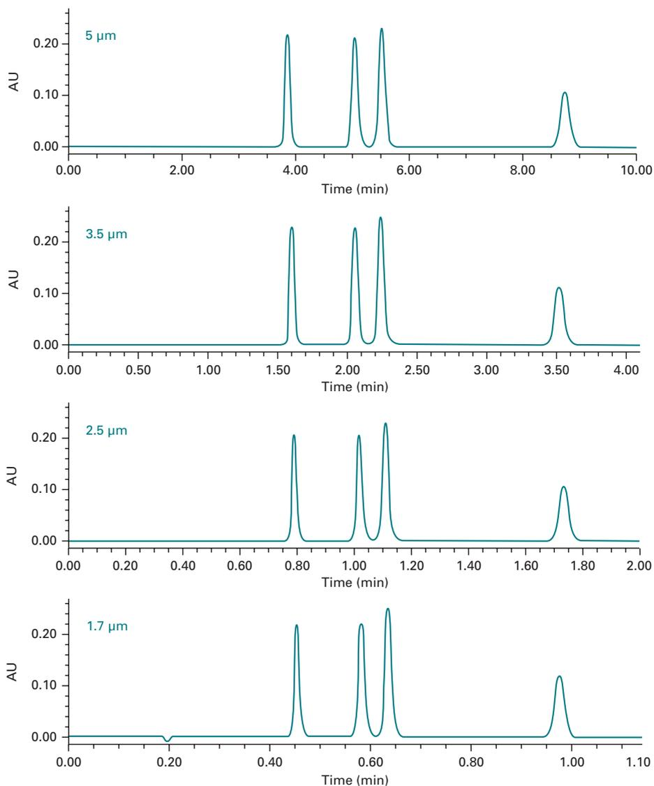
Fig 11.7 Chromatograms showing the influence of particle size on the resolution and elution time of four analytes in an HPLC system demonstrating the time advantages of the pressure-tolerant sub-2  $\mu\text{m}$  ACQUITY UPLC system. (Reproduced by permission of Waters Corporation, UK.)
