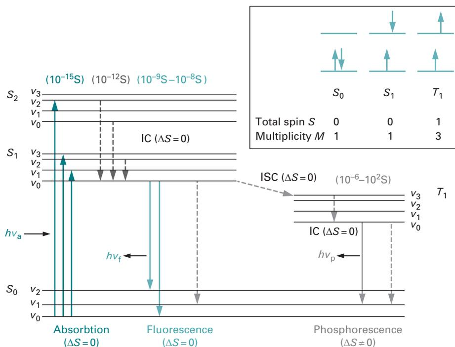
Fig. 12.8 Jablonski diagram. Shown are the electronic ground state ( $S_0$ ), two excited singlet states ( $S_1, S_2$ ) and a triplet state ( $T_1$ ). Vibrational levels ( $\nu$ ) are only illustrated exemplarily. Solid vertical lines indicate radiative transitions, dotted lines show non-radiative transitions. The inset shows the relationship between electron configurations, total spin number  $S$  and multiplicity  $M$ .
