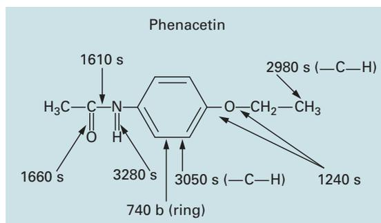
Fig. 13.3 FT-IR spectrum of phenacetin, the historically first synthetic fever reducer to go on the market. Bands at the appropriate wavenumbers ( $\text{cm}^{-1}$ ) are shown, indicating the bonds with which they are associated, and the type (s, stretching; b, bending).
