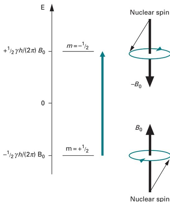
Fig. 13.7 Energy levels of a proton in the magnetic field  $B_0$ . The nuclear spin of a nucleus is characterised by its magnetic quantum number  $m$ . For protons,  $m$  can only adopt  $+\frac{1}{2}$  and  $-\frac{1}{2}$ . The corresponding energies are calculated by  $-m\gamma h/(2\pi)H_0$ , where  $\gamma$  is a constant characteristic for a particular nucleus,  $h$  is the Planck constant, and  $H_0$  is the strength of the magnetic field  $B_0$ .
