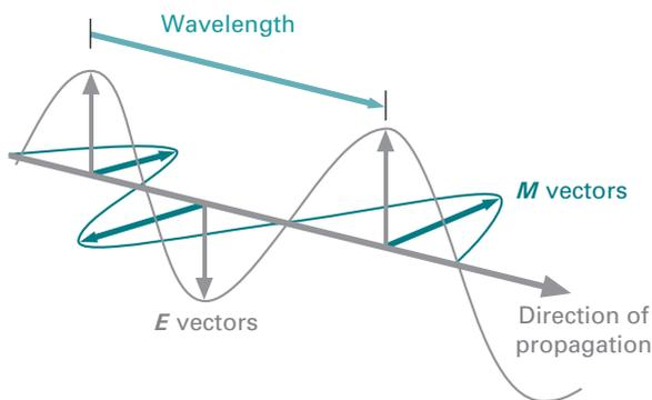
Fig. 12.1 Light is electromagnetic radiation and can be described as a wave propagating transversally in space and time. The electric ( $E$ ) and magnetic ( $M$ ) field vectors are directed perpendicular to each other. For UV/Vis, circular dichroism and fluorescence spectroscopy, the electric field vector is of most importance. For electron paramagnetic and nuclear magnetic resonance, the emphasis is on the magnetic field vector.
