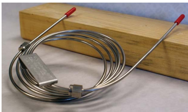
Figure 12.23 Typical example of a packed column for gas chromatography. This column is made from stainless steel and is 2 m long with an internal diameter of 3.2 mm. The packing material in this column has a particle diameter of 149–177 \mu\text{m} . To put this in perspective, beach sand has a typical diameter of 700 \mu\text{m} and the diameter of fine grained sand is 250 \mu\text{m} .
