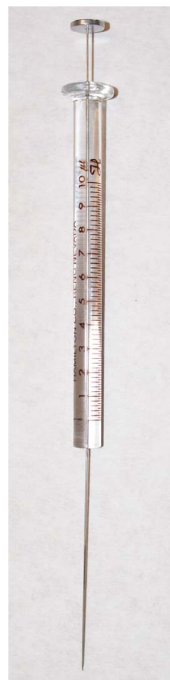
Figure 12.29 Example of a syringe for injecting samples into a gas chromatograph. This syringe has a maximum capacity of 10 μL with graduations every 0.1 μL.
