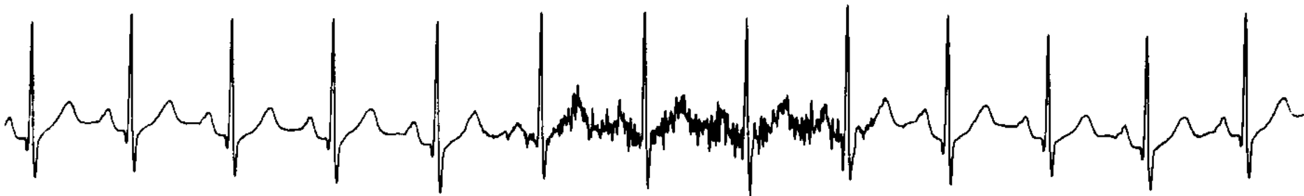
(b) Electromyography interference on the ECG
