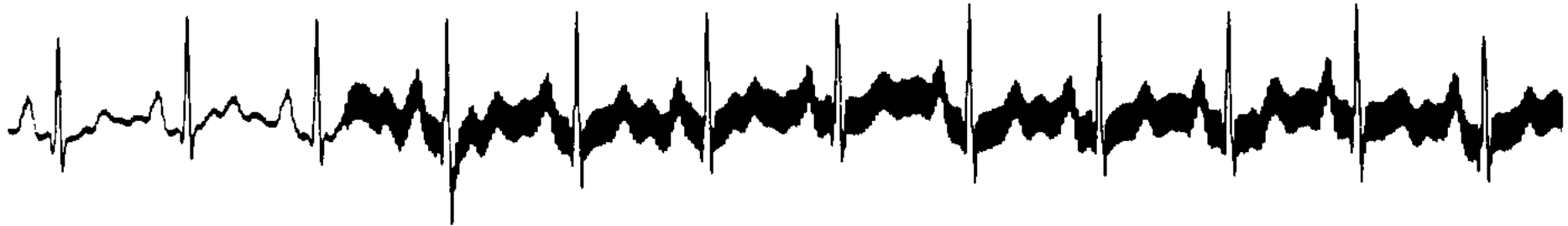
(a) 60-Hz power-line interference on the ECG
