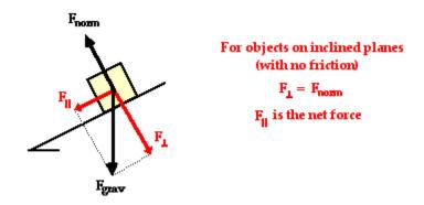
The task of determining the magnitude of the two components of the force of gravity is a mere manner of using the equations. The equations for the parallel and perpendicular components are:
