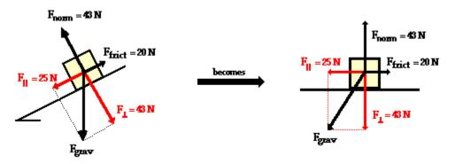
Once the force of gravity has been resolved into its two components and the inclined plane has been tilted, the problem should look very familiar. Merely ignore the force of gravity (since it has been replaced by its two components) and solve for the net force and acceleration.
