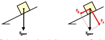
The force of gravity can be resolved into two components. Together, these two components replace the affect of the force of gravity.
