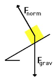
The first peculiarity of inclined plane problems is that the normal force is <u>not</u> directed in the direction opposite the direction of the force of gravity. But this is only because the object is no longer on horizontal surfaces. The truth about normal forces is not that they are always upwards, but rather that they are always directed perpendicular to the surface that the object is on.
