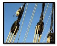
4. If a rope is guided over a pulley, the direction of the tension force is changed but the magnitude is still the same everywhere
