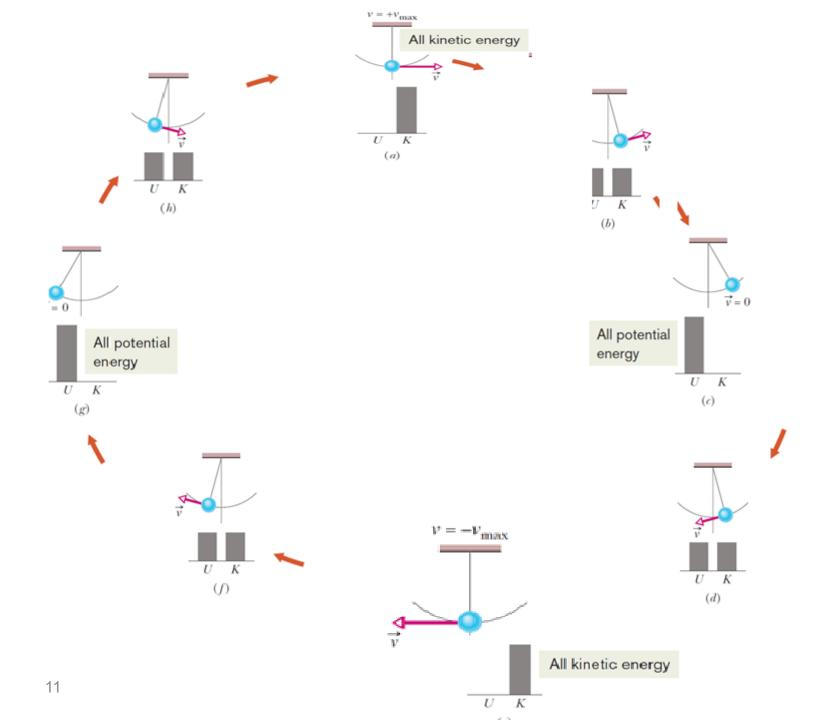
principle of conservation of mechanical energy can be applied:
