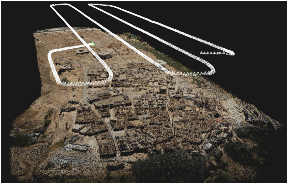
Dense 3D point cloud of Ad Diriyah using UAV images
