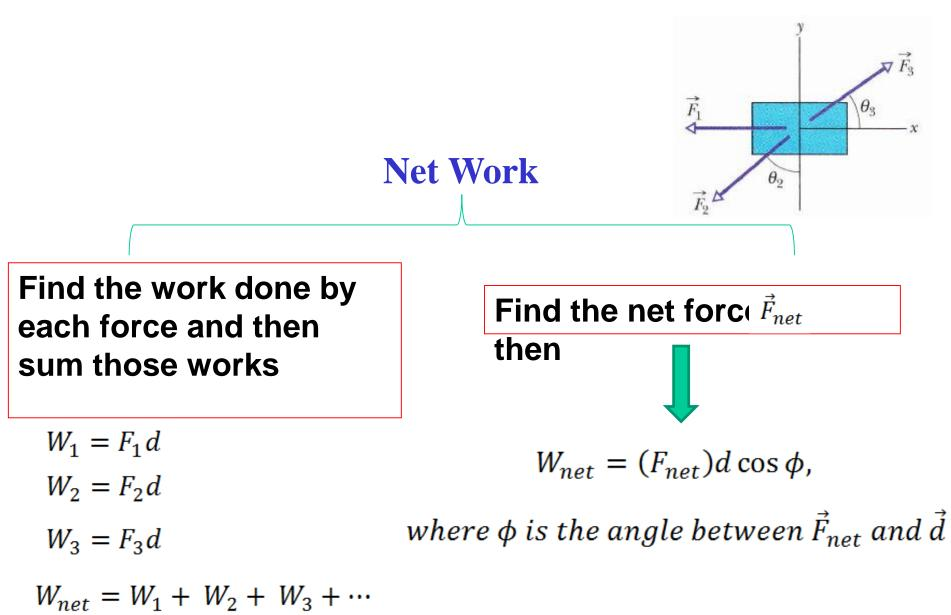
Net Work: If we have several forces acting on a body there are two methods that can be used to calculate the net work  $W_{net}$
