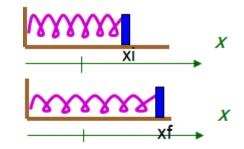
Work  $W_s$  is positive if the block ends up closer to the relaxed position (x = 0) than it was initially. It is negative if the block ends up farther away from x = 0. It is zero if the block ends up at the same distance from x = 0.
