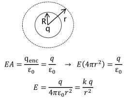
Therefore, the electric field just about the surface of the sphere, r = R, is
