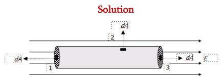
As shown above, we divided the cylinder into 3 faces. Through face 1, we note that the area is anti-parallel to the electric field (angle is 180). Therefore
