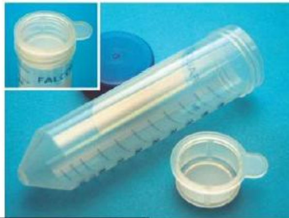
Fig. 12.8. Cell Strainer. Disposable polypropylene filter and tube for straining aggregates from primary suspensions (BD Biosciences). Can also be used for disaggregating soft tissues (see also Fig. 12.13).
