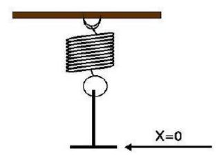
The equilibrium position of a hanging spring can be changed by adding weights to the hanger. The force on the spring stretches it by a distance x given by Hook's law F=-kx. This situation is shown in the figure below.
