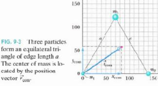
$x_{\text{com}} - \frac{1}{M} \sum_{i=1}^{3} m_i x_i = \frac{m_1 x_1 + m_2 x_2 + m_3 x_3}{M}$   $= \frac{(1.2 \text{ kg})(0) + (2.5 \text{ kg})(140 \text{ cm}) + (3.4 \text{ kg})(70 \text{ cm})}{7.1 \text{ kg}}$   $= 83 \text{ cm} \qquad (Answer)$ and  $y_{\text{com}} = \frac{1}{M} \sum_{i=1}^{3} m_i y_i = \frac{m_1 y_1 + m_2 y_2 + m_3 y_3}{M}$   $= \frac{(1.2 \text{ kg})(0) + (2.5 \text{ kg})(0) + (3.4 \text{ kg})(120 \text{ cm})}{7.1 \text{ kg}}$   $= 58 \text{ cm}. \qquad (Answer)$
