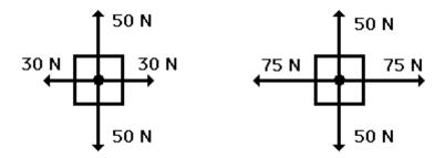
If an object is at equilibrium, then the forces are balanced. *Balanced* is the key word that is used to describe equilibrium situations. Thus, the net force is zero and the acceleration is  $0 \text{ m/s}^2$ . Objects at equilibrium must have an acceleration of  $0 \text{ m/s}^2$ . This extends from Newton's first law of motion. But having an acceleration of  $0 \text{ m/s}^2$  does not mean the object is at rest. An object at equilibrium is either ...
