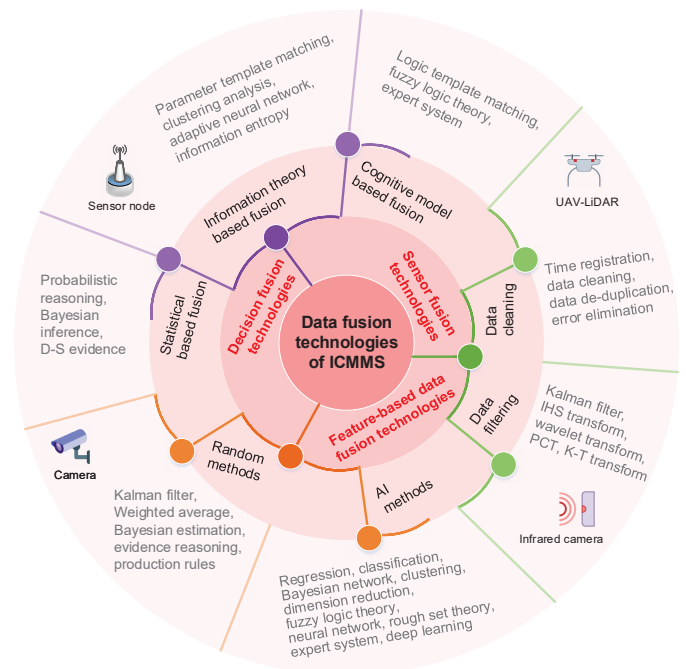
FIGURE 3. Classification of sensor fusion, feature-based data fusion and decision fusion technologies.
