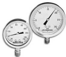
FIGURE 3-2 Two basic pressure gages. Dresser Instruments, Dresser, Inc. Used by permission.
