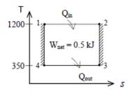
Solution A Carnot cycle with specified temperature limits is considered. The maximum pressure in the cycle, the heat transfer to the working fluid, and the mass of the working fluid are to be determined.
