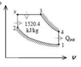
Solving for  $T_x$  we get  $T_x = 250$  K which is impossible. Therefore, constant specific heats at room temperature turned out to be an unreasonable assumption in this case because of the very high temperatures changes involved.
