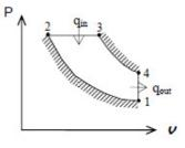
(b)  $q_{\rm in} = h_3 - h_2 = c_p (T_3 - T_2) = (1.005 \text{ kJ/kg} \cdot \text{K})(1818.8 - 909.4)\text{K} = 913.9 \text{ kJ/kg}$
