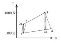
$$w_{s,C,in} = h_{2s} - h_1 = c_p (T_{2s} - T_1) = (1.005 \text{ kJ/kg} \cdot \text{K})(610.2 - 300)\text{K} = 311.75 \text{ kJ/kg}$$
