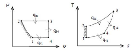
$$T_{2} = T_{l} \left(\frac{P_{2}}{P_{l}}\right)^{(k-1)/k} = (300 \text{ K}) \left(\frac{1000 \text{ kPa}}{100 \text{ kPa}}\right)^{0.4/1.4} = 579.2 \text{ K}$$
