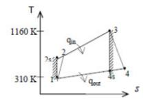
$$P_{r_2} = \frac{P_2}{P_1} P_{r_1} = (8)(1.5546) = 12.44 \longrightarrow h_{2s} = 562.58 \text{ kJ/kg} \text{ and } T_{2s} = 557.25 \text{ K}$$
