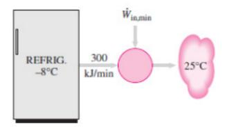
Solution The refrigerated space and the environment temperature for a refrigerator and the rate of heat removal from the refrigerated space are given. The minimum power input required is to be determined.
