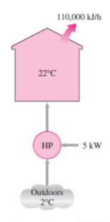
Solution A heat pump maintains a house at a specified temperature. The rate of heat loss of the house and the power consumption of the heat pump are given. It is to be determined if this heat pump can do the job.
