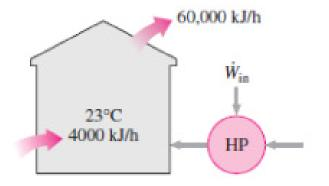
Solution The rate of heat loss, the rate of internal heat gain, and the COP of a heat pump are given. The power input to the heat pump is to be determined.
