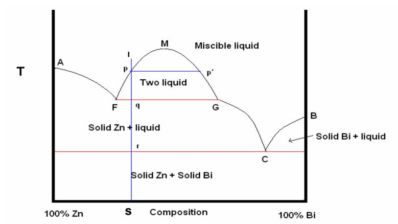
Example Zn-Bi system, which gives the above diagram. This diagram shows partially immiscible over certain composition range.
