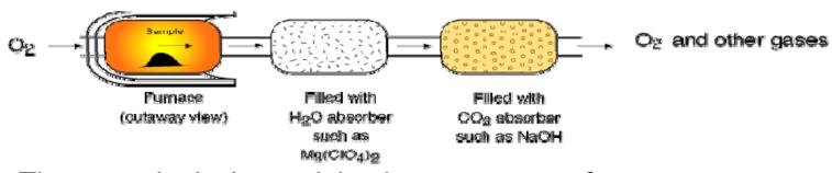
The sample is burned in the presence of excess oxygen which converts all the carbon to carbon dioxide and all the hydrogen to water.
