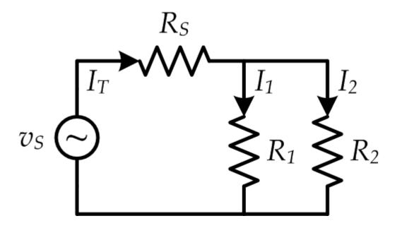
$$I_1 = I_T \frac{R_2}{R_1 + R_2}$$
