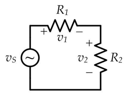
$$v_1 = v_s \frac{R_1}{R_1 + R_2}$$
