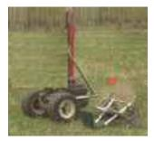
you can begin recording ground motion from the geophones at the instant the slug or shell hits the ground.
