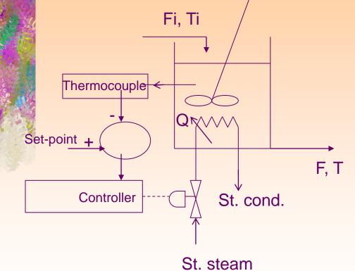
A thermocouple measures the temperature of the fluid in the tank. Then this temperature is compared with the desired value yielding a deviation
